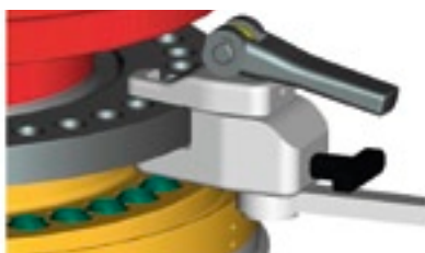
2 Dismantling/installation tool for Die Shells
