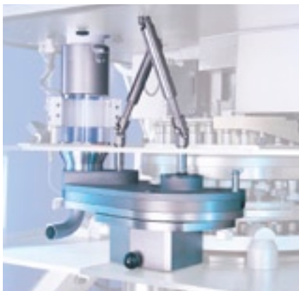
Double paddle feeder with 2 independent drive motors.
