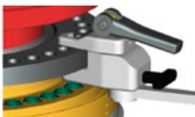
2 Dismantling/installation tool for Die Shells
