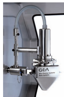
Measuring head and data analysing equipment discretely mounted onto the rotating blending head assembly.
